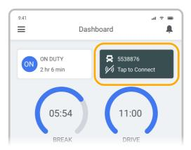
Use Tap to Connect bar to connect to your vehicle. The device will attempt to connect to selected vehicle ELD via Bluetooth. ELD bar will change from red to orange: Pairing.
